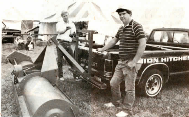
Kelly Baird (operating winch) and Steve Seymour teamed up to develop this 3-pt. hitch for pickups.
