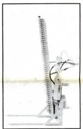
Pto-powered vertically-mounted sickle bar is pushed down into bale by a single hydraulic cylinder.
