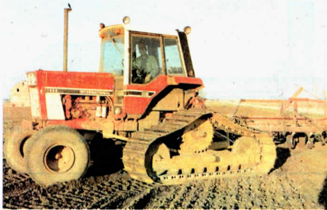
Caterpillar D-5 half tracks replace rear wheels on International 1586.
