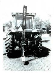
Each soil sample is deposited in 30-sample container as it's taken.
