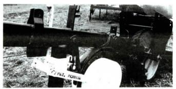
Gauge wheels for each row are mounted on a 2 by 2-in. stub welded to planter frame. Cable ties to central "one lever" system for adjusting all row units simultaneously.
