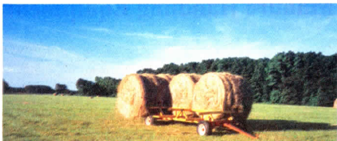
Bale-carrying frame fits any existing running gear. Each bale is contained in a cradle so it won't fall off as cattle feed.
