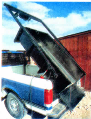
A 1 1/2 cu. yard dump box lifts in and out of pickup bed, letting you use pickup as a dump truck.
