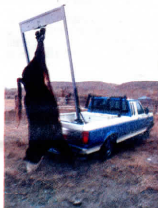
Boom handles loads up to 1,200 lbs. Can be used to transport dead cattle.
