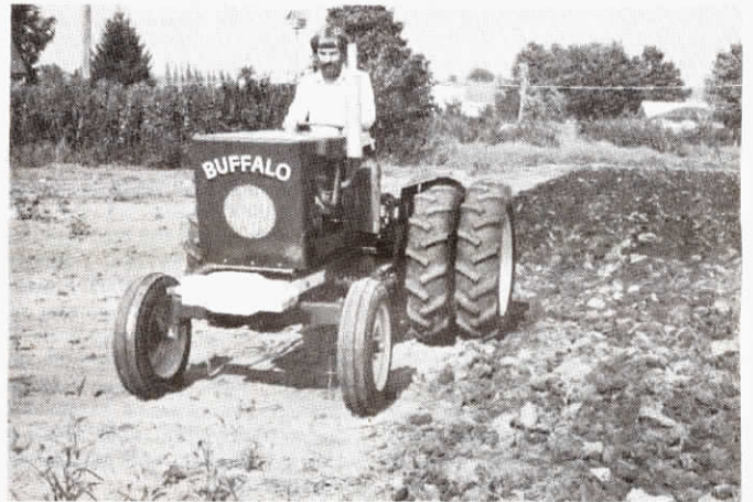
The 25 hp Buffalo tractor can be outfitted with duals for field work. Vern Schield, manufacturer, saw a need for moderately priced tractor that would fit between available garden tractors and larger diesel models.
