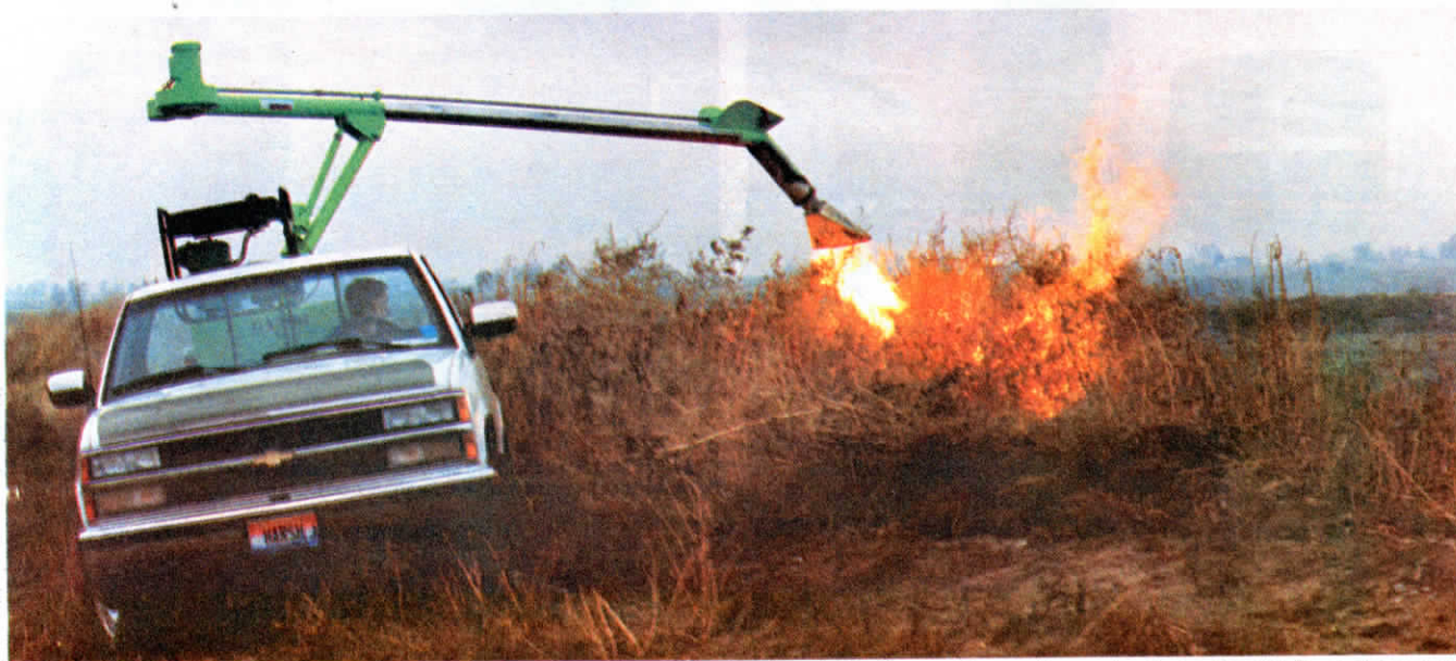
Diesel-fired flame thrower lets you burn off weeds from comfort of your air-conditioned pickup cab. Steel burner tube mounts on center pivot and is rotated by electric motors.
