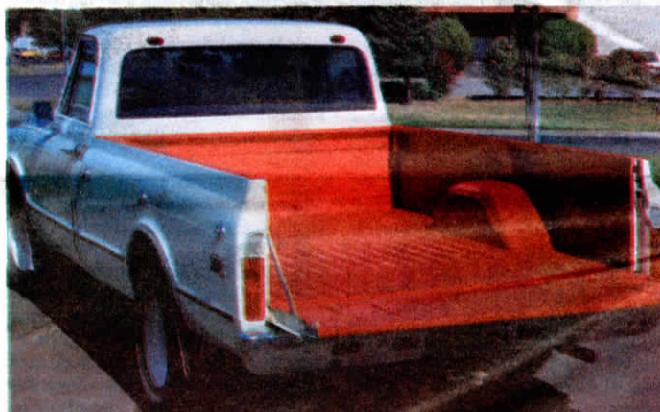
Polyurethane spray-on liner fits contours of pickup bed like a glove.
