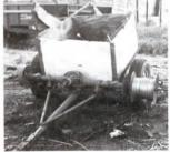
A splined pto shaft mounts on the input shaft to the drive axle. It's pto-driven by the tractor pulling the trailer. The wire winder is used to wind up wire using the pto and to unwind wire by driving along the fence line and allowing the spool to unwind freely.
