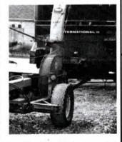
box drive shaft, shift the chopper feed rolls into neutral, and start up the pto. When the box is empty, disconnect the forage box shaft and head back to the field. It saves lots of time spent hooking and unhooking wagons and one tractor does it all. I use the same setup for fenceline feeding."
