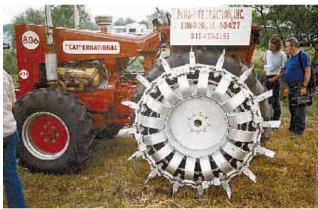
Fold-out cleats are 10 in. wide and 5 in. high. They mount on 2-WD, 4-WD, or front wheel assist tractors with 26, 32, 38, or 42-in. dia. wheels.
