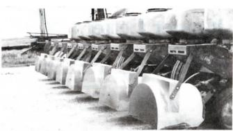
For several years I have been selling no-drift plastic spray hoods set up with 3 tips to band spray growing crops. Now I am also taking the same hood and cutting it in the center so it's 17 in. long and mounting it on the back of row crop planters to protect the band from wind, letting farmers more accurately band spray while planting.
