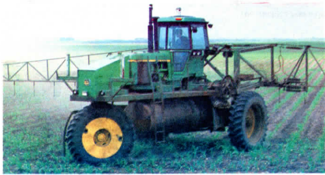
Tractor could be converted back to normal use by unbolting it from sprayer frame.
