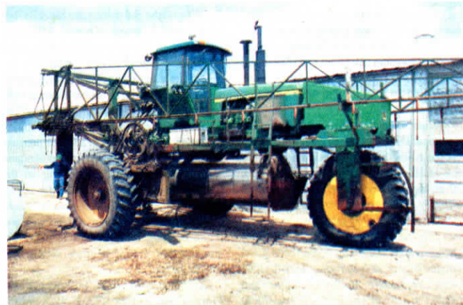
Rear wheels are chain-driven by sprockets bolted to extensions on tractor's rear axle.
