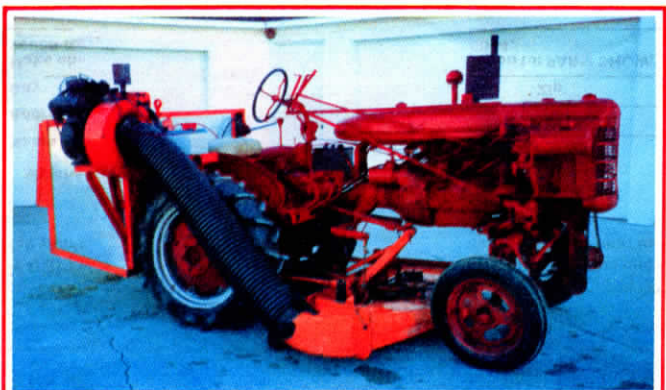
Tractor could be converted back to normal use by unbolting it from sprayer frame.
