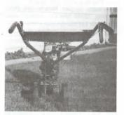
"After the sod is cut, I just use a small 4-in. wide spade to lift the sod, drop the pipe in under the sod, and then set the sod back into the trench. Then you just have to set up sprinkler heads.
