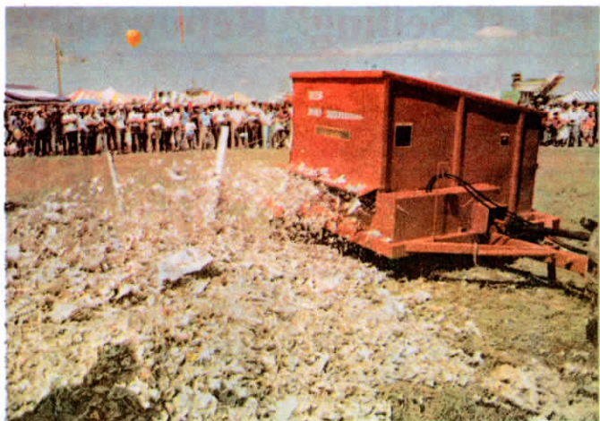
Chopped newspapers are thrown out the side or in a windrow alongside the chopper.
