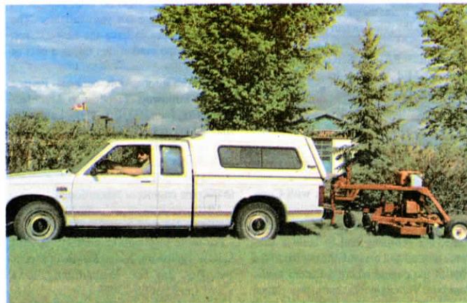
One person can hitch the mower up behind a pickup and tow it at highway speeds. A cable lets you control the engine choke from the vehicle.
