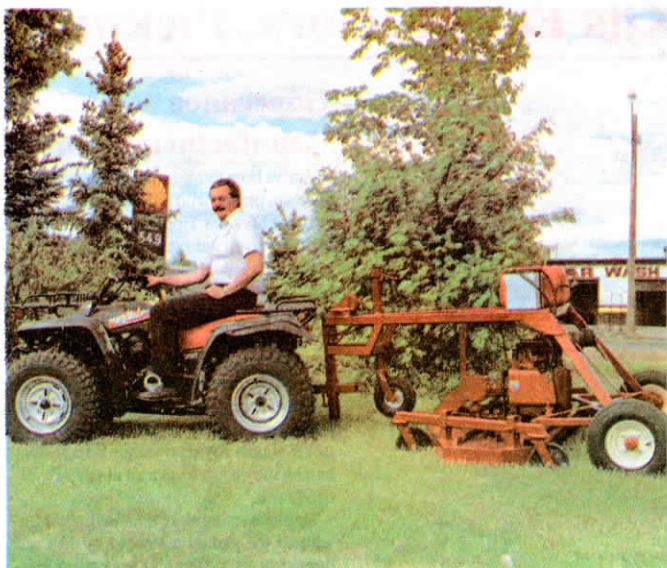
The 60-in. wide "Grass Guzzler" is powered by its own 18 hp Kohler engine and can be towed behind any vehicle equipped with a ball hitch, including ATV's.
