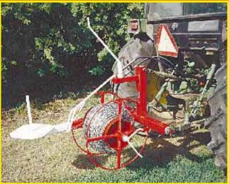
New-style wire roller lets you roll up wire quickly and easily.
