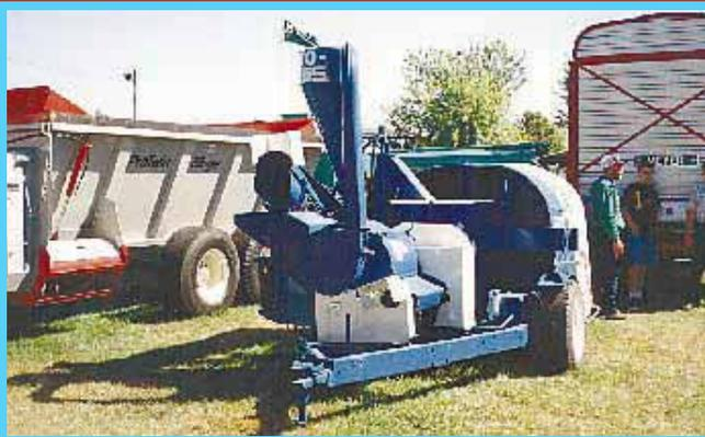
Bagger is built from refurbished 21-in. wide, 20-in. dia. Gehl grinder-mixer.
