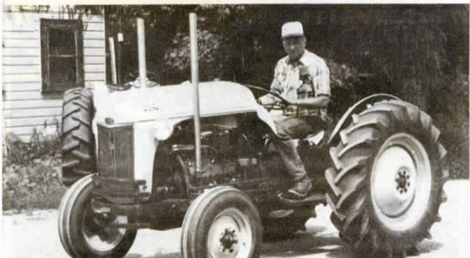
This 1949 8N Flathead V-8 conversion tractor was equipped with the same engine used in the early Ford V-8 cars of the late 1940's and early 1950's.
