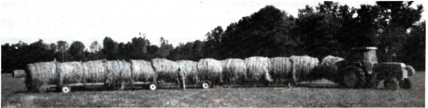
Photo shows two log bale haulers hooked together. Albright often adds one more trailer behind to haul as many as 19 bales.
