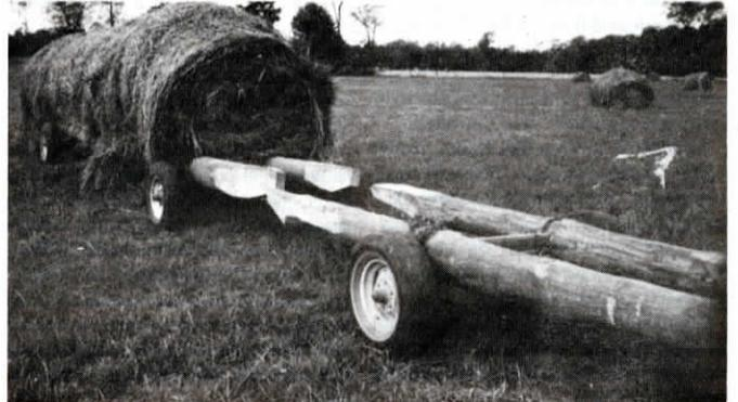
Albright puts spacer bars between the logs and chains them to the trailer chassis. He notches the ends of the logs so they won't touch when turning.
