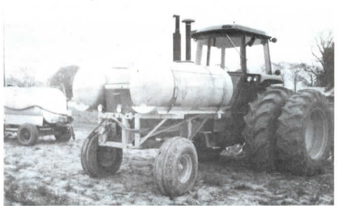
Each 200-gal. tank is supported by a special mounting system. Chemical hoses connect in front so Chailland doesn't have to unhook them to swing tanks out.
