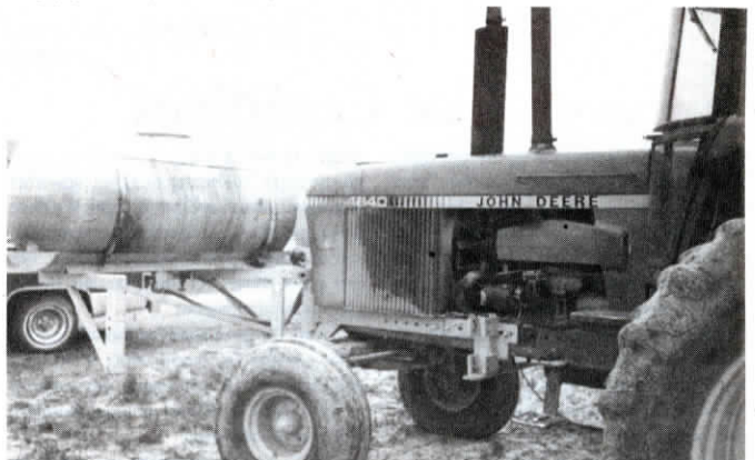
Tanks can be pivoted forward empty or full by pulling two pins and swinging tanks out. Rack, made out of angle iron and tubing, bolts directly to tractor frame.
