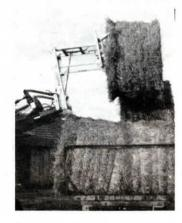
"This bale stacker is unique because you can mount it on the front-end of any tractor without adding hydaulies to power its cylinders. It's also the only bale stacker that'll pick bales up horizontally and set them back down vertically for storage or transport," says Francois Vasseur, Faucheux Industries.
