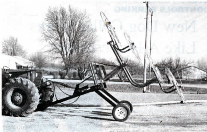
Cart lets you rake with a smaller tractor and allows the rake to more closely follow the ground contour, and also eliminates fishtailing around corners.
