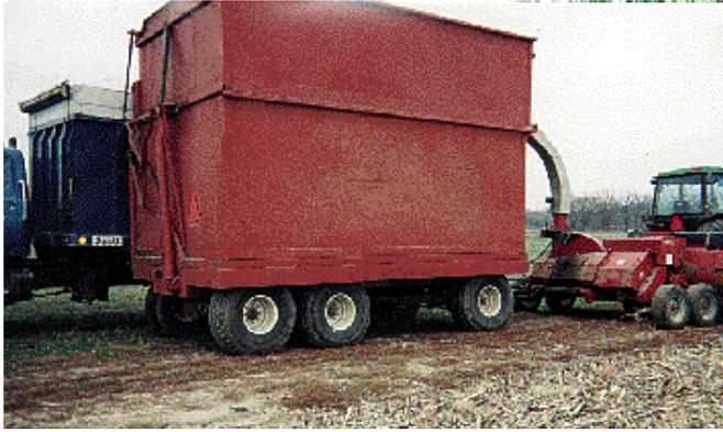
The wagon, 12 ft. high, 9 ft. wide and 15 ft. long, mounts on 18-ton running gear.
