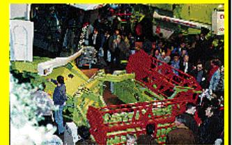
One new product Claas demonstrated at the show was a new folding grain head that makes transport easier on narrow roads.
