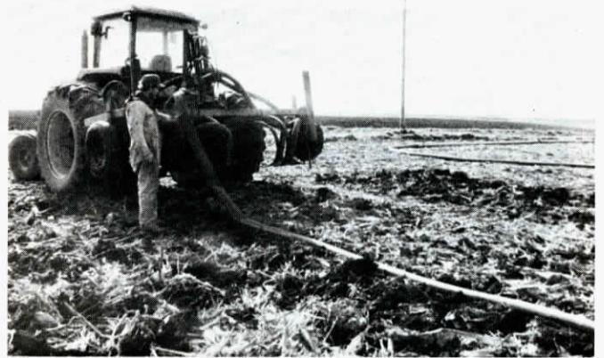
A 4½ in. flexible hose carries manure to tractor-mounted injector.
