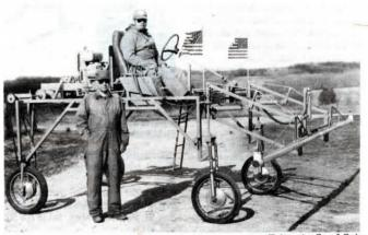
The "crop mop" machine is fitted with Yamaha motorcycle axles and wheels.
