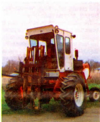
The original header lift controls are used to raise and lower the forklift mast.
