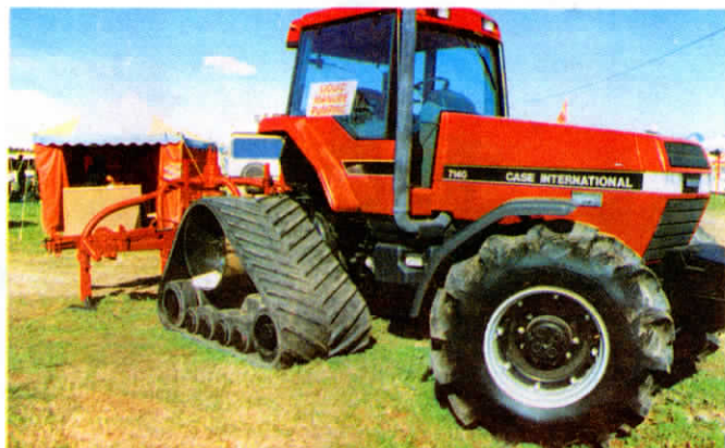
Gilbert & Riplo's 36-in. wide rubber tracks mount in place of the rear wheels on most any tractor or combine.
