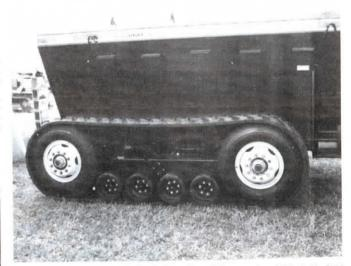
Holt-Refakis, a Caterpillar dealer in Columbus, Ohio, recently exhibited this Gehl manure spreader fitted with rubber tracks built by Mason Dixon Farms. The company, which operates throughout the state of Ohio, will work with customers to fit the compaction-cutting tracks to most any trailing farm equipment. Contact: FARM SHOW Followup, Holt-Refakis, 5252 Walcott Ct., Columbus, Ohio 43228 (ph 614 878-2287).
