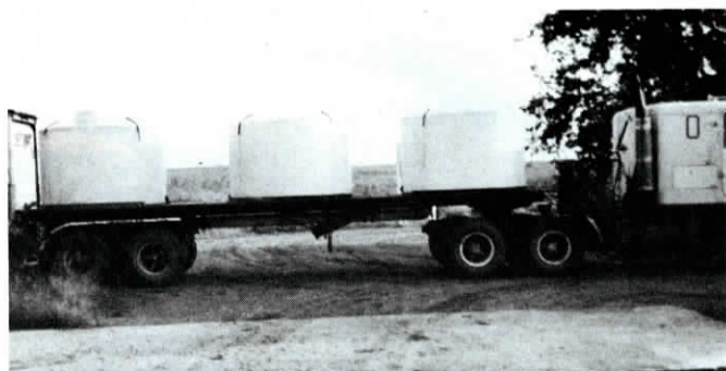
An 8-in. pipe, running beneath the flatbed, connects all three 1,500-gal. tanks.
