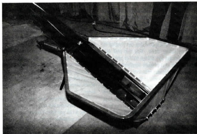
By flipping a lever, you can collapse hopper to slip it under a semi-truck or hopper bottom bin.
