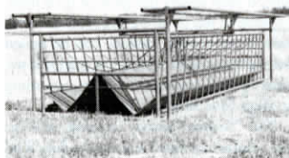
When the 4 bales in feeder are gone, you pull cord to dump bales on one of side racks into feeder.
