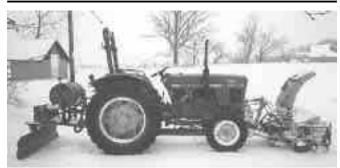
After reading the many great ideas in each issue of FARM SHOW, I'd like to pass along an idea of my own. The photo shows my 33 hp. Deere 1050 tractor equipped with a snowblower on front and a blade on back. The blower is driven by a 21 gpm Prince pto-mounted pump drawing oil from a reservoir tank carried on top of the rear blade.
