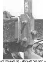
and then used big U-clamps to hold them to the bar. The vertical adjustment screws are still in place on the bracket. (John Rathjen, Rt. 1, Ft. Calhoun, Neb. 68023)
