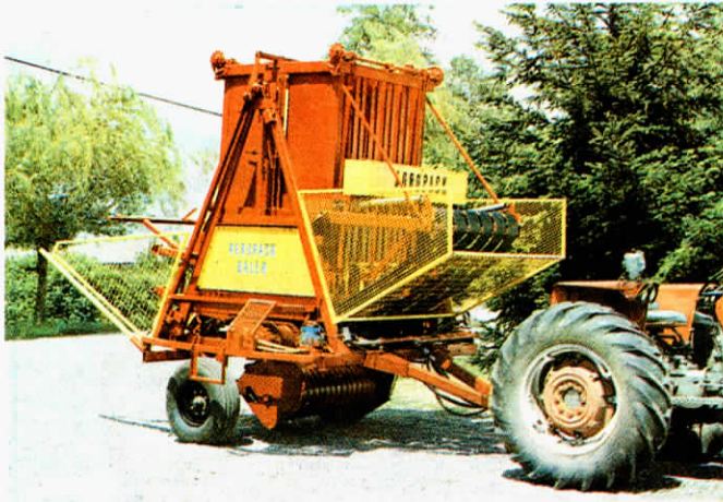
Bale chamber swings back and forth like a bell in operation, making a layered bale about the size and density of a round bale.
