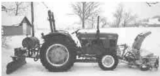
After reading the many great ideas in each issue of FARM SHOW, I'd like to pass along an idea of my own. The photo shows my 33 hp. Deere 1050 tractor equipped with a snowblower on front and a blade on back. The blower is driven by a 21 gpm Prince pto-mounted pump drawing oil from a reservoir tank carried on top of the rear blade.
