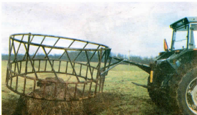
Two-in-one bale handler also puts feeder ring around bale.
