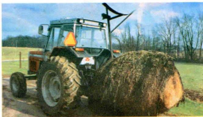
To move a bale, ring handler raises up out of the way via hydraulic cylinder.
