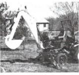
We built this mobile backhoe from scratch. It mounts on its own wheels and can be pulled by a small garden tractor. Every piece was made out of sheet steel except for the hydraulic controls. It works as well as any commercial rig. (Clarence & Bruce Cole, 7 Fallon Dr., Westport, Mass. 02790)
