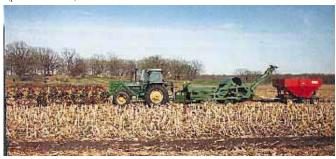
Resch first got into the down corn retrieval business 12 years ago when he put this big rig together. Rake wheels up front pulled loose ears and residue into a windrow that was picked up by a rock picker-type rig behind the tractor. It separated out stalks and rocks from the corn and augered the ears into a trailing wagon. Resch savs the machine worked great but was too big to transport easily, and required a separate operation to shell the corn.
