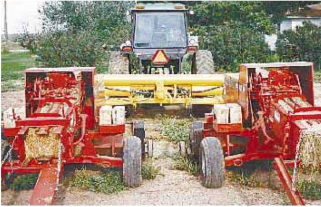
Hydraulic-powered hitch is used to pull two Case-IH 8545 balers behind a Deere 4040. Balers hitch to hydraulically-operated arm on each end.
