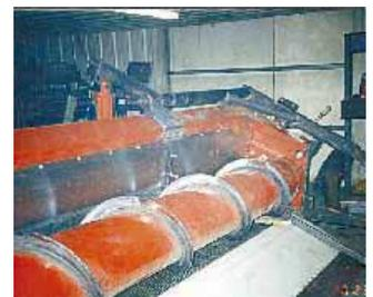
Flighting on header cross auger is downsized to better handle the flow of residue and crop material into combine.
