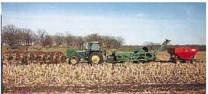
Resch first got into the down corn retrieval business 12 years ago when he put this big rig together. Rake wheels up front pulled loose ears and residue into a windrow that was picked up by a rock picker-type rig behind the tractor. It separated out stalks and rocks from the corn and augered the ears into a trailing wagon. Resch says the machine worked great but was too big to transport easily, and required a separate operation to shell the corn.
