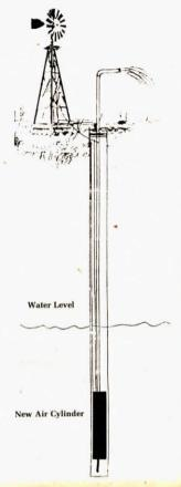
cylinder. He belt-drives his compressor off the windmill shaft.
