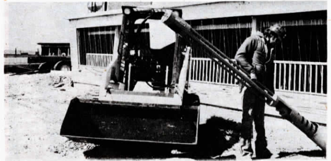
Entire Sludge Eliminator, motor and all, weighs only 130 lbs. and is only 6½-in. in dia.
