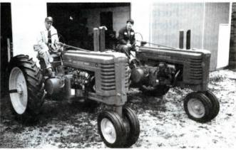
There are now two John Deere "A's" powered by V-8 diesel engines and both were converted by John Jones of Odon Machine, I read the article about Odon, Indiana. Jones in FARM SHOW a year ago (Vol. 16, No. 6) that described how he had replaced the 2-cyl. gas engine in his 1944 Deere "A" with an Oldsmobile 350 diesel. It caught my eye because I had just bought a 1950 "A' that had sat outside for many years. The
