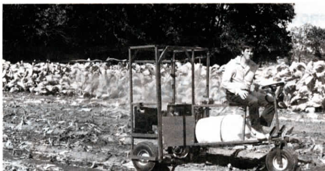
Self-propelled sprayer, designed for smaller farms, adapts to 36 to 46-in. rows.
