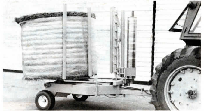
Vermeer's bale-wrapper picks bale up off ground and then spins it for wrapping.
