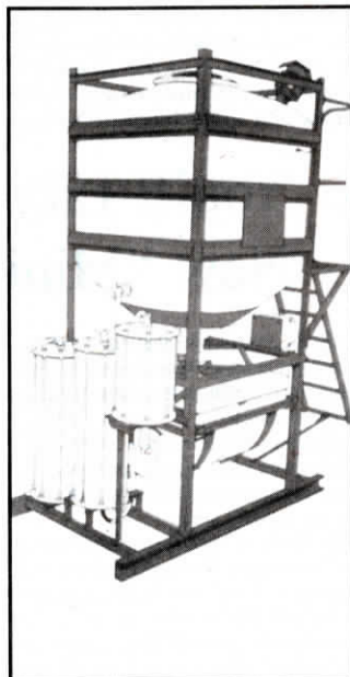
Leftover spray material gravity flows from 265 gal. holding tank, through sand filter and through two carbon filters, leaving only a few pounds of sludge to be taken to an approved disposal facility.
