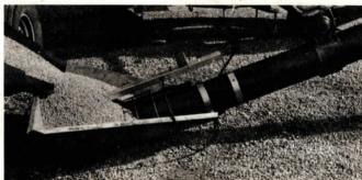
Auger attachment "grounds out" powering tractor when grain flow stops.
