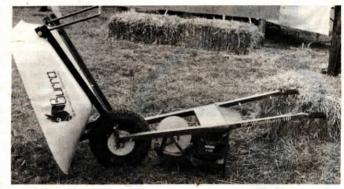
Only the dumpbed on new powered wheelbarrow tips up to empty a load.
