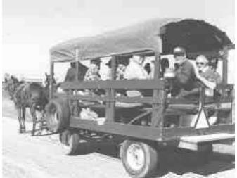
The wagon is equipped with the running gear out of a 1938 Ford car and fitted with 15-in. wheels.
