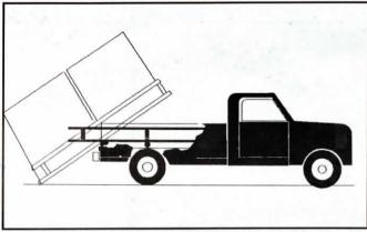
Bale cradle mounts on pickup bed. To unload, drive backward and then hit brakes. Cradle rolls back and tips over back edge of pickup. Pull forward to clear bales.
