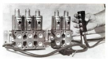
New push button controlled hydraulic outlet "multiplier" lets you run up to five hydraulic circuits from a single set of outlets.
