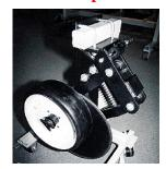
"The greater the angle of the blade, the more soil is thrown outward. Most gauge wheels are only 2 in. wide. We made our gauge wheel 4 inches wide so that it can run on top of the coulter-disrupted soil which isolates the coulter and keeps it operating at a consistent depth."
