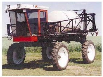
The Frieds' sprayer is powered by a 400 cu. in. short block V-8 engine that's been souped up to  $220\,\mathrm{hp}.$
