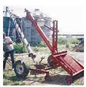
Auger raises up for transport. Note light for night work.
