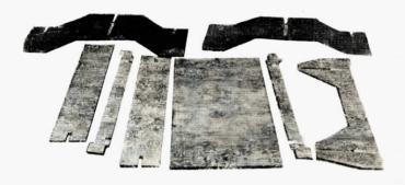
Entire table is made from one 4 by 8 sheet of 3/4 in. plywood.
