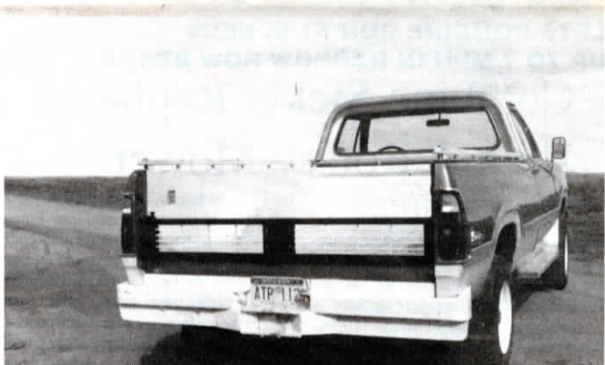
Gate offers an unobstructed view of trailers while towing or backing up and doesn't block air flow which boosts mileage.
