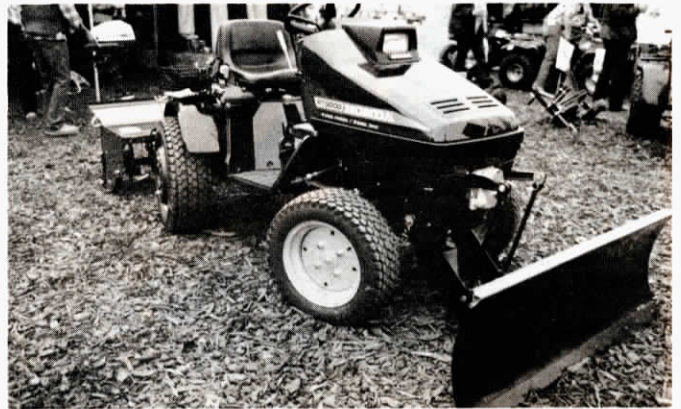
Rear steering wheel "kicks in" automatically on short turns.
