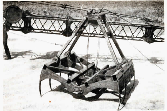
Teeth on the 2,500 lb. bucket grab up to 14 hay bales at a time.
