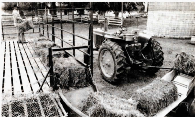
Conveyor carries bales to front of wagon and into fiberglass chute that drops them into elevator.
